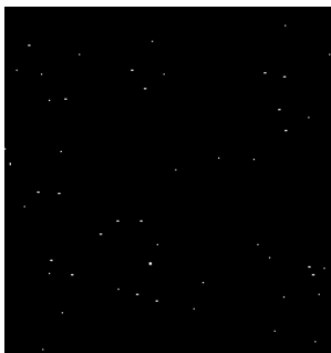
Fig. 17.— Here we display our Bad Pixel Mask for the Infrared Camera with bad pixels shown in white. Bad pixels have unstable gain properties often incorrectly arbitrarily high or low numbers of counts which could potentially throw off your photometry. After defining the bad pixel mask, we only use the good pixels in our subsequent calculations.
