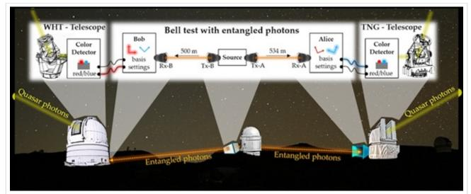
This graphic shows the experimental setup used to test the freedom-of-choice loophole. Researchers produce two entangled photons (middle) and shoot them in opposite directions toward detectors located at each telescope. The telescope then use ancient quasar light to determine which properties of the photons to measure.
