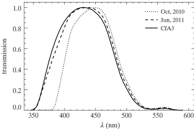
**Figure 3.** C12 *B* passbands measured before (dotted) and after (dashed) the 2011 May bakeout, showing the blueward shift caused by the bakeout. The CfA3 synthetic *B* passband (solid) agrees fairly well with the post-bakeout C12 *B* passband.
