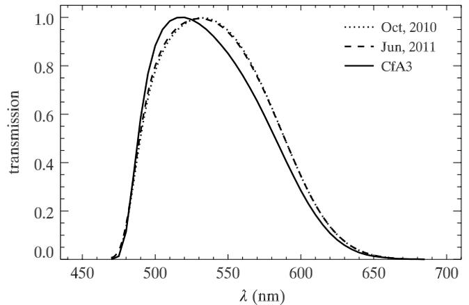
**Figure 2.** C12  $V$  passbands measured before (dotted) and after (dashed) the 2011 May bakeout are highly consistent with each other and in reasonable agreement with the CfA3 synthetic  $V$  passband (solid).
