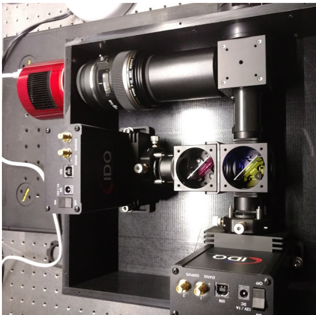
FIG. 3. Photo of our astronomical random-number generator in the laboratory with the lid off and dichroic mirrors exposed.
